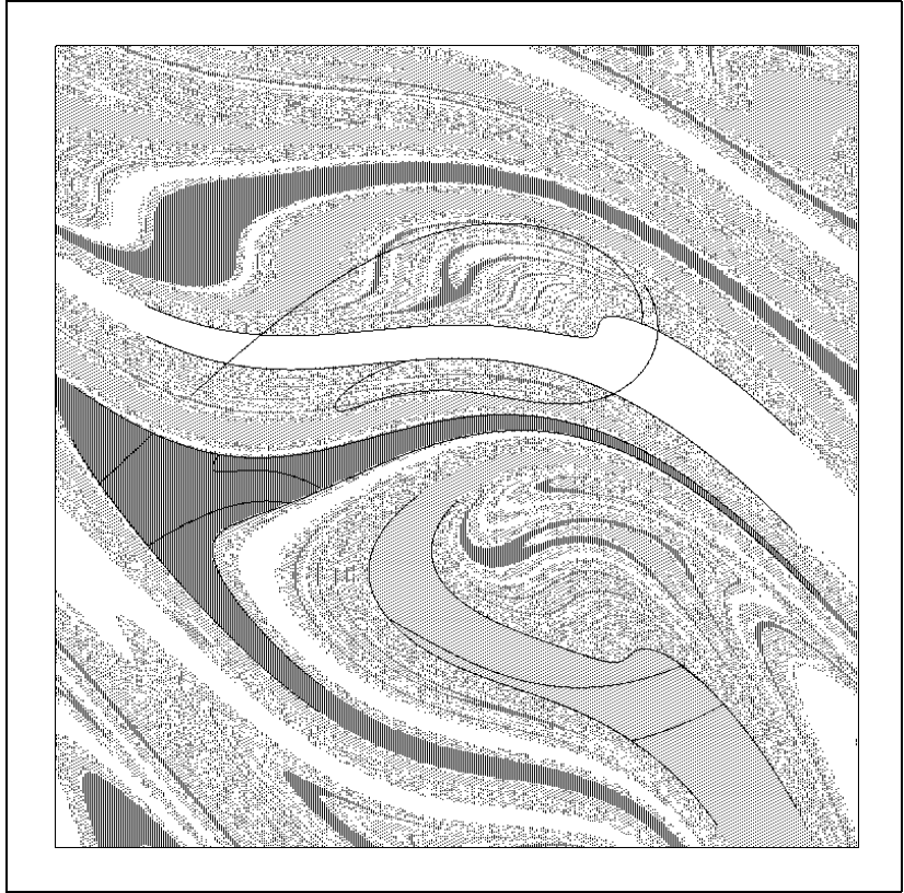
Figure 10.30 Three basin cells for the time- 2\pi map of the forced, damped pendulum.
