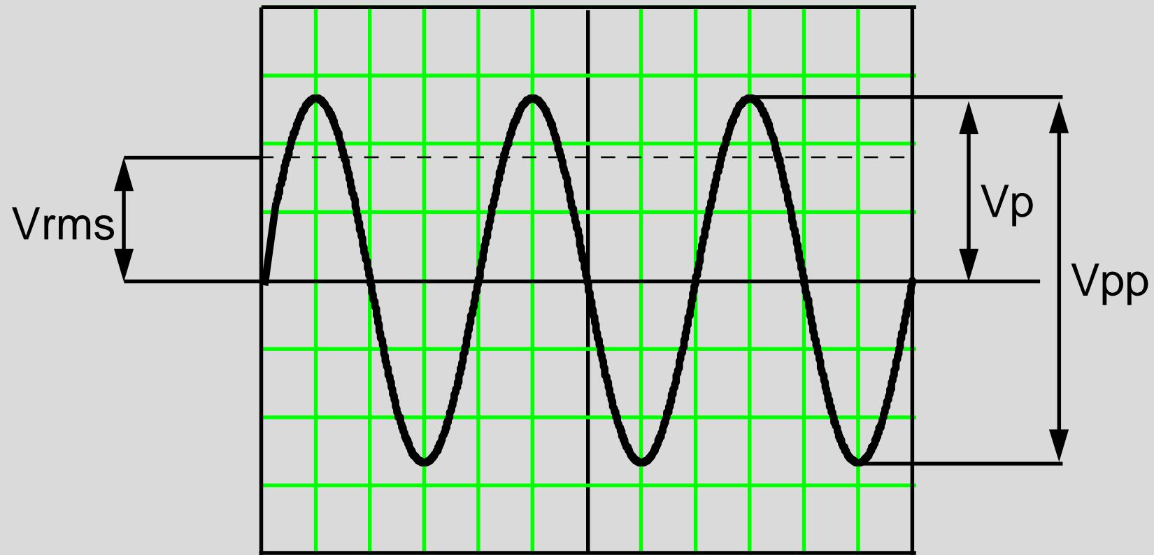
$$V_{rms} = V_p \cdot .707 \text{ (Sine wave)}$$
