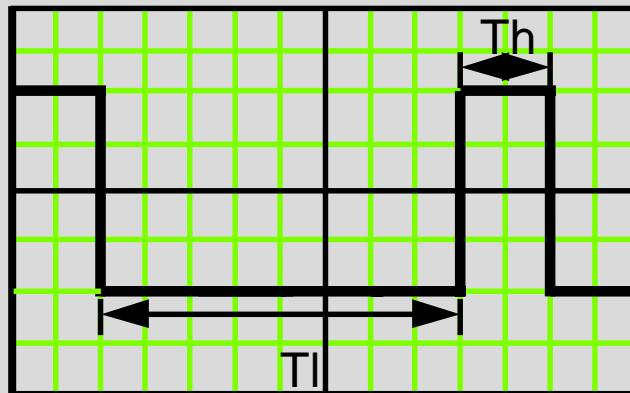
Less than 50% (Pulse Train)  $T_l \neq T_h$
