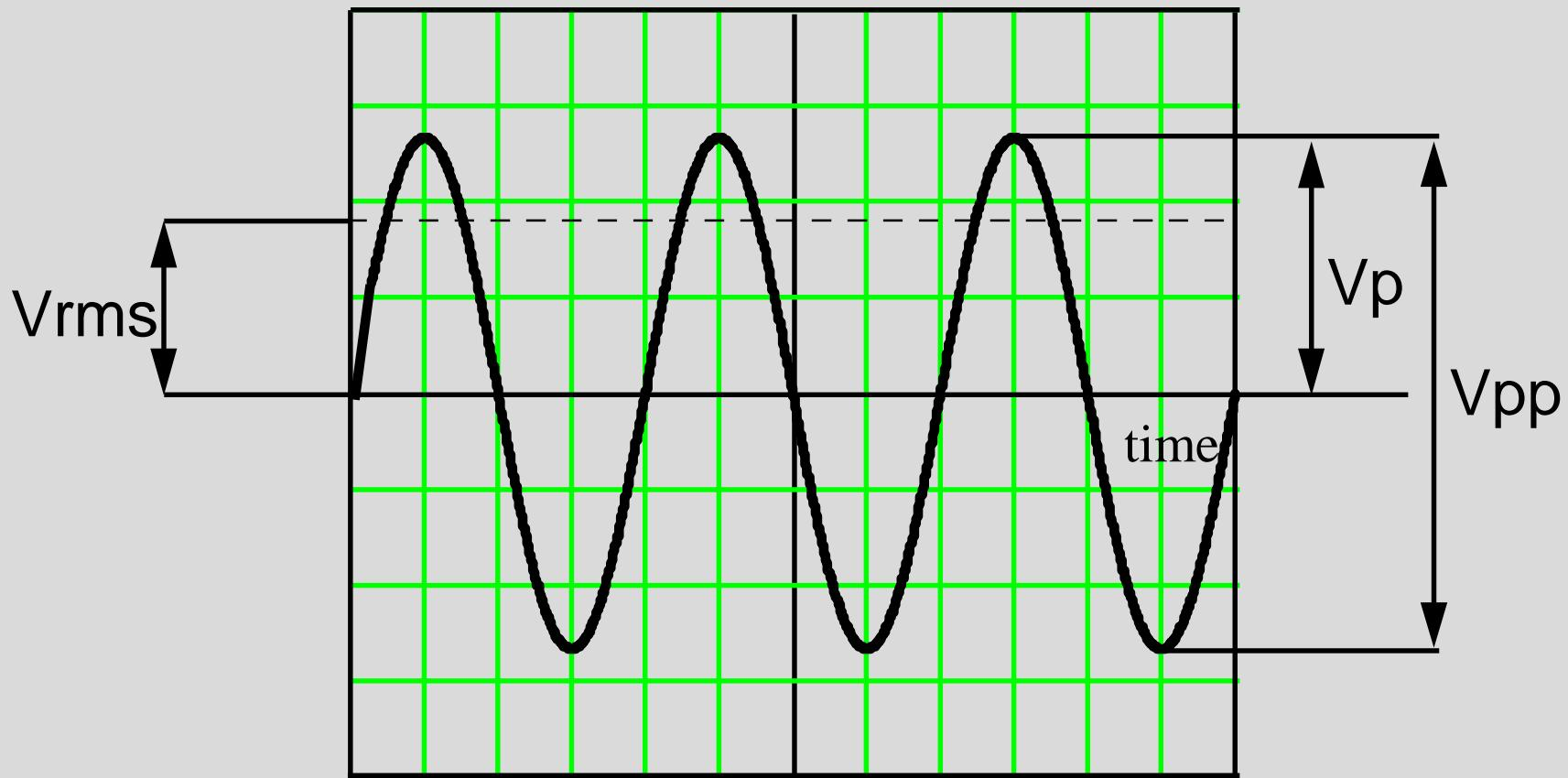
$$V_{rms} = 0.707 V_p \text{ (Sine wave)}$$
