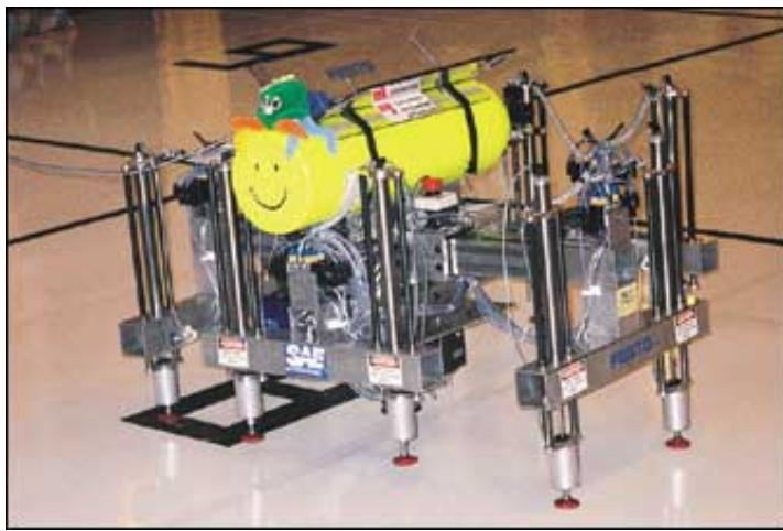
This robot, designed by a team from the University of Quebec at Rimouski, sports a whimsical grin as it completes the "dash" event. The remote-controlled walking machine features eight independent legs that operate pneumatically.
