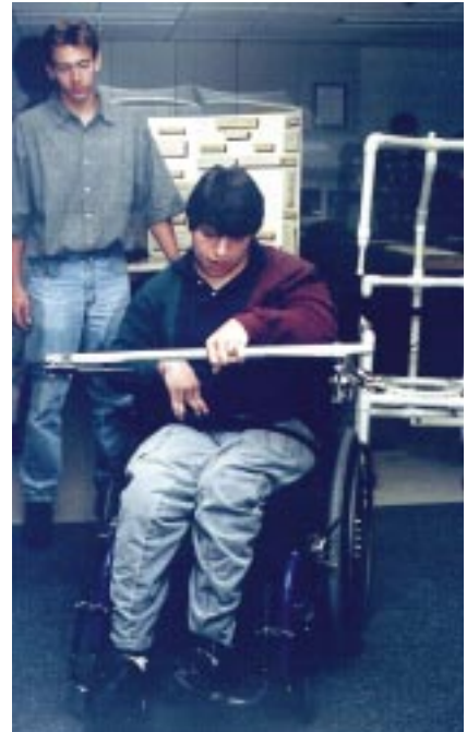
At CU, first-year engineering students design and build assistive devices for disabled clients. This gearing system, created by a four-student team, allows its delighted owner to propel his own wheelchair by pushing down on the lap bar.
