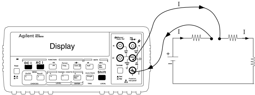
The input resistance of the ammeter is  $0.1 \Omega$  for the 1A and 3A ranges, and  $5 \Omega$  for the 10 mA and 100 mA ranges. This means that it will not load the circuit and result in a large measurement even for most resistance values (100 k $\Omega$  to 2  $\Omega$ ).
