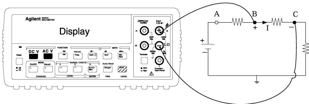
The input resistance of the voltmeter is  $10\text{ M}\Omega$ . This means that it will not load the circuit and result in a large measurement error if the resistances are  $300\text{ k}\Omega$  or smaller (see lab report assignment).
