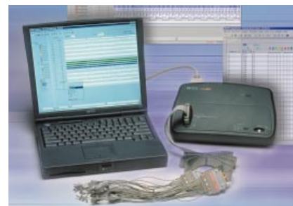
The LogicWave Logic Analyzer: 34 channels with 100 MHz state and 250 MHz timing analysis; 128 K sample depth per channel. Download the interface software free from our website.
