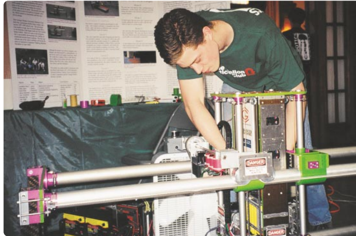
Jonathan Hurst, a third-year student at Carnegie Mellon University, makes a final adjustment to his team's walking machine, Jim2, which placed first overall in this year's decathlon. Jim2 walks using five actuators moving two independent frames so the main mass of the body is in continuous motion. This allows Jim2 to conserve energy and attain high speeds.
