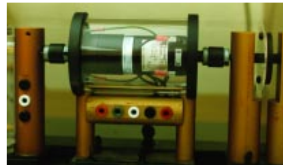
Amplifier/Motor/Potentiometer was built in-house using a variety of components.
