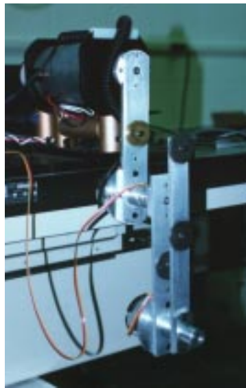
This Pendubot – a doubly underactuated planar robot – is currently used as part of an instructional experiment in the lab. Students develop a control algorithm and an electronics interface with a digital signal processing board to make the mechanical system (Pendubot) balance.
