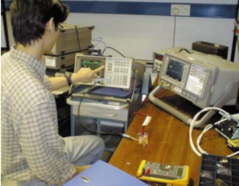
A University of Surrey student measures the noise sidebands of the oscillator he is designing for his final - year undergraduate project.
