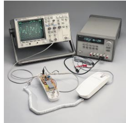
An HP 54600B Oscilloscope displays dialer output for digit 8 at speaker.
