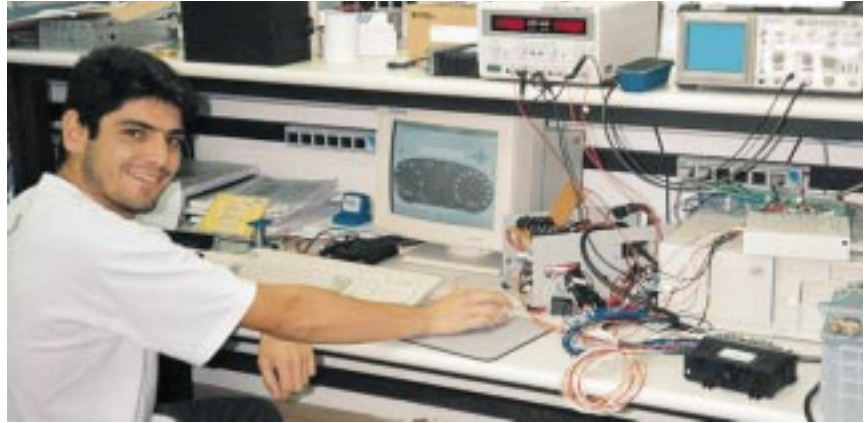
At a Universidade Estadual de Campinas lab in Brazil, performing research for Magneti Marelli of Italy, a student works on an automated test for automotive instrument panels.
