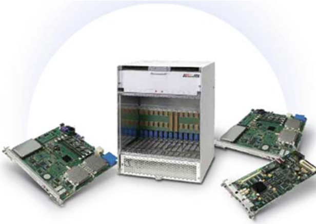
Fig. 13.13 ATCA chassis and blades
