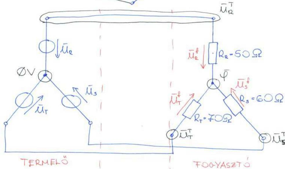
$$\begin{aligned} \bar{U}_R &= 230V \\ \bar{U}_S &= 230 e^{-j120^\circ} V \\ \bar{U}_T &= 230 e^{j120^\circ} V \end{aligned}$$
