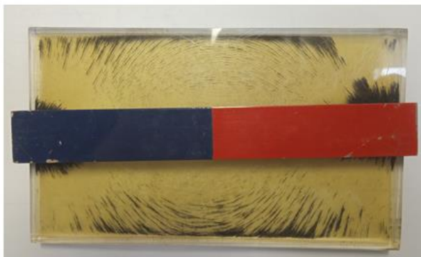
Fig.14. Magnetic field of permanent (bar) magnet
