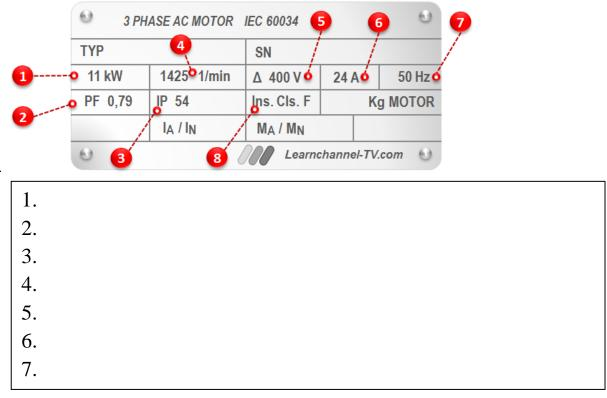
B. Calculate the torque of the motor (use the cos  $\phi$  value of 0.79). Calculation required!
