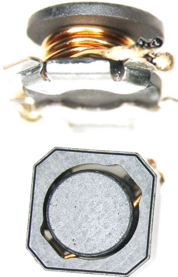
Fig. 4.27. The microscopic photo of the inductor
