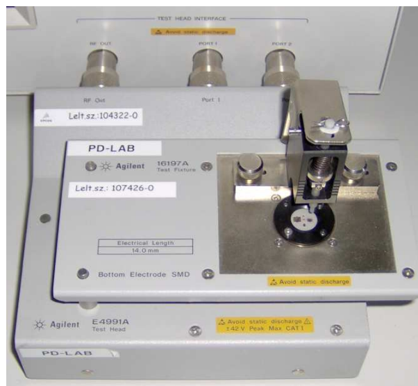
Fig. 4.9. Agilent 16197A SMD Test Fixture
