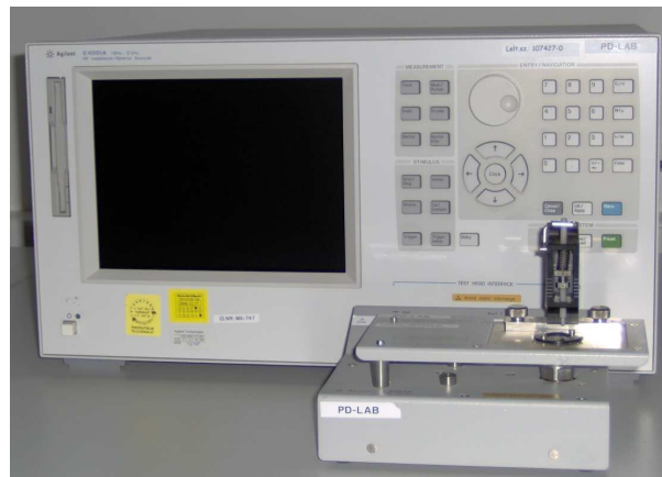
Fig. 4.8. Agilent E4991A RF impedance and material analyzer
