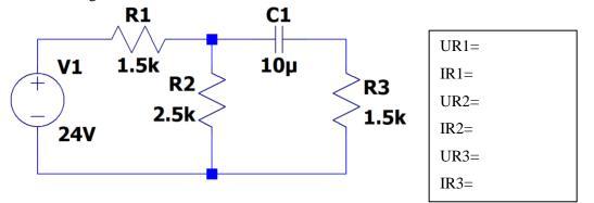
4. Calculate the voltage and current of all the resistors. Only the values are not enough!
